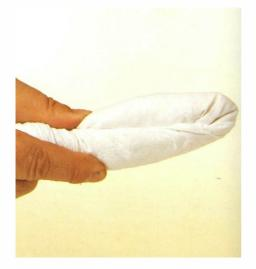
5. To charge the rubber, open out the linen to expose the wadding, then pour a small amount of polish onto the wadding. With practice you will be able to judge the correct quantity. Note: if the rubber is too dry, it will not run smoothly over the surface.
