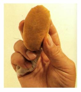
4. The rubber is complete when the tail is completely twisted. For a smaller, more intricate polishing job, make a smaller version of the rubber to suit.
