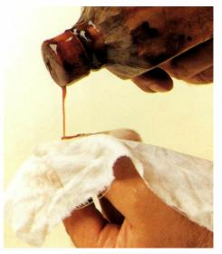
6. Refold the linen around the wadding. Squeeze the tail to apply pressure to the wadding to force the polish through the linen. The more you tighten the tail, the more polish will flow.
