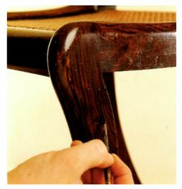
2. Apply dark brow n stain to match the grain of the simulated rosew ood, using a fine brush to replicate the pattern.
