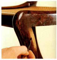
1. Apply a base coat of light brow n stain mixed to match the existing colour. Charge a rubber with polish and apply a thin layer..
